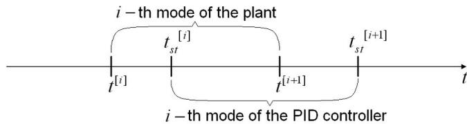
Fig. 1. Time intervals of plant and PID controller
