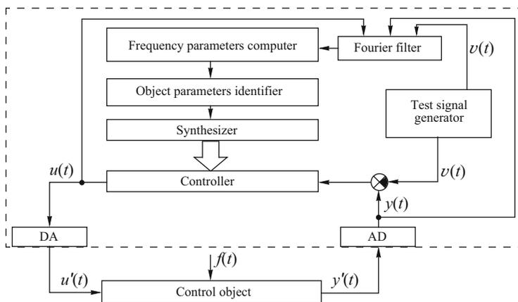
Fig. 1. Structural scheme of an adaptive controller.
