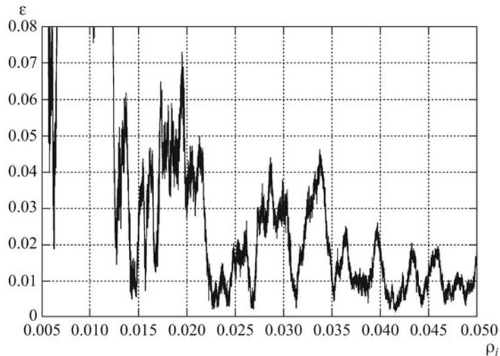
Fig. 8. Dependence of relative error in the coefficients of the identified object on the test signal amplitudes (enlarged).
