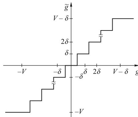
Fig. 2. Static characteristic of the quantizer.
