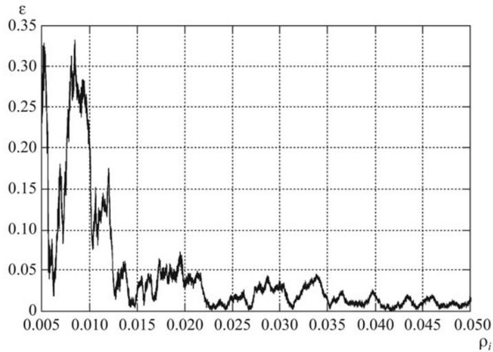
Fig. 7. Dependence of relative error in the coefficients of the identified object on the test signal amplitudes.
