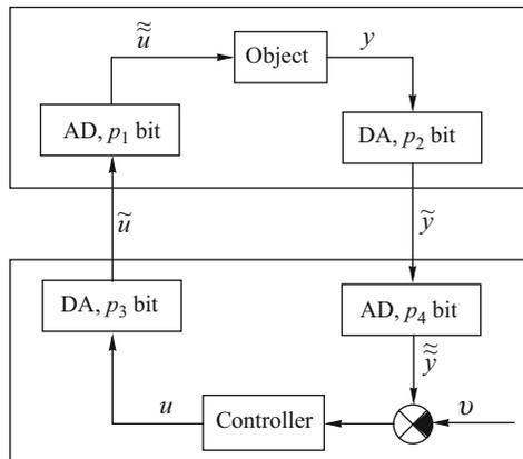
Fig. 3. The testbed structure with DA and AD converters.
